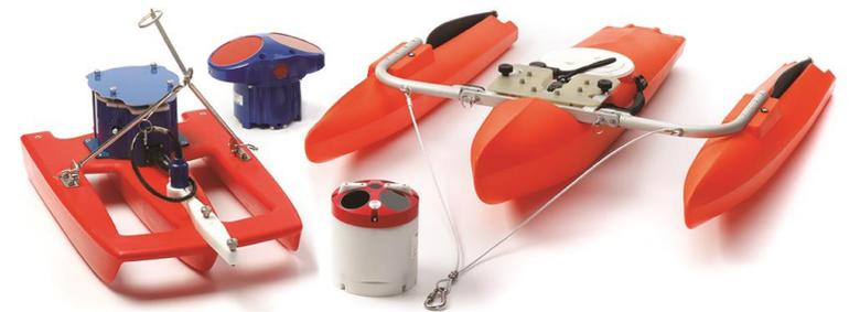
An Acoustic Doppler Current Profiler (ADCP) is a type of sonar that measures and records **water current** velocities over a range of depths via a single instrument. This data is calculated to measure river flow and discharge.
