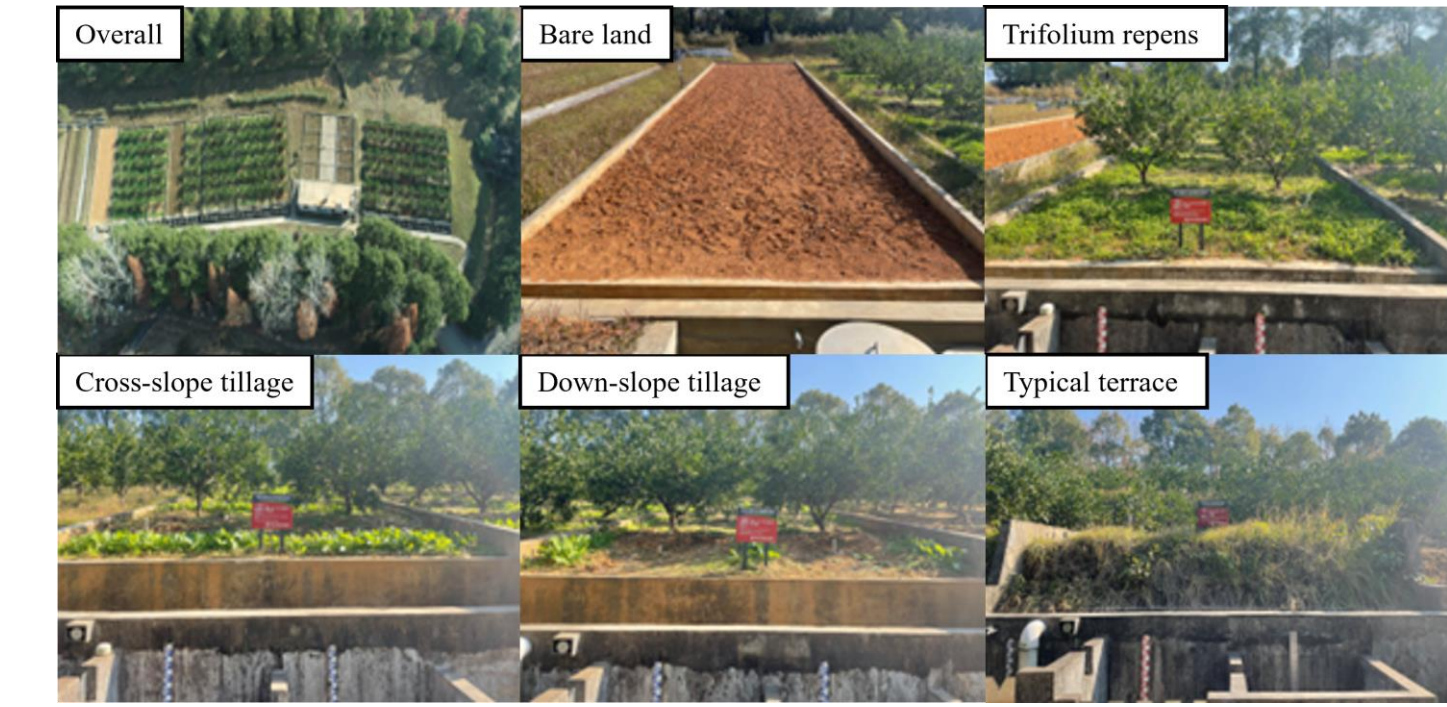
Figure. (A) Overall view of the experimental environment; (B) Runoff plot without any vegetation cover; (C)-(F) Runoff plots covered with Trifolium repens , typical terrace, cross-slope tillage, and down-slope tillage, respectively.
