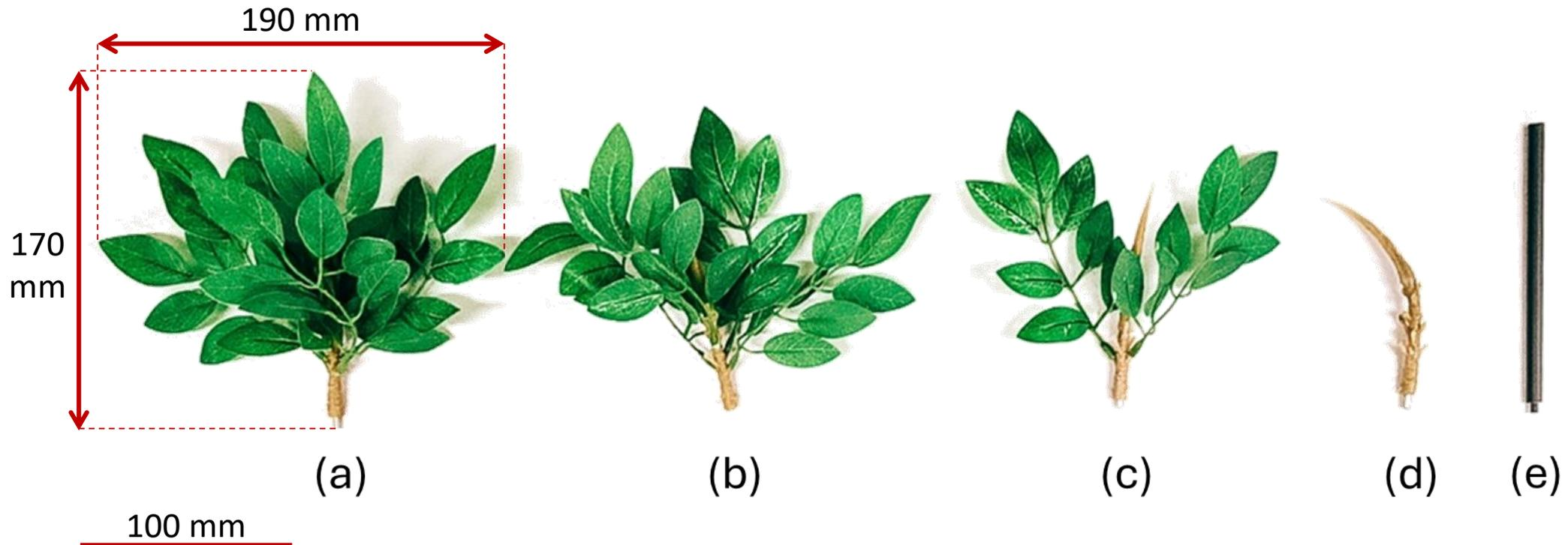
Switching from rigid cylinder arrays to realistic plant forms: (a) 6 branches, (b) 4 branches, (c) 2 branches, (d) single stem, and (e) 8 mm cylinder.
