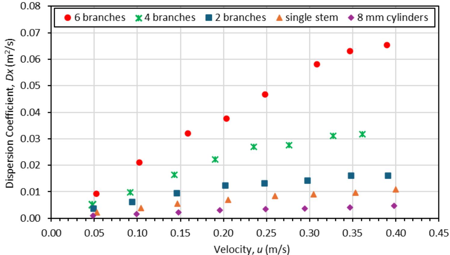
$D_x$  increases with velocity and vegetation density; denser setups show stronger dispersion, while sparse or cylinder setups show lower  $D_x$ .
