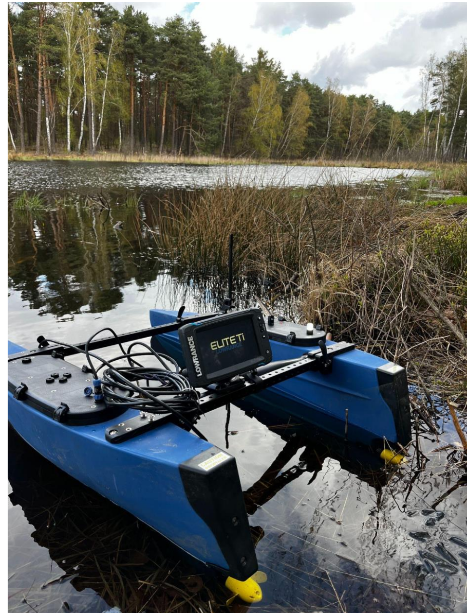
Unmanned radio-controlled catamaran boat with electric motors propulsion equipped with sonar and GPS receiver
