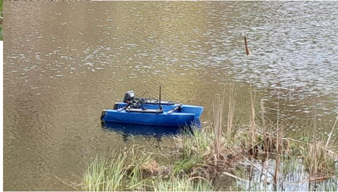
Unmanned radio-controlled catamaran boat with electric motors propulsion equipped with sonar and GPS receiver
