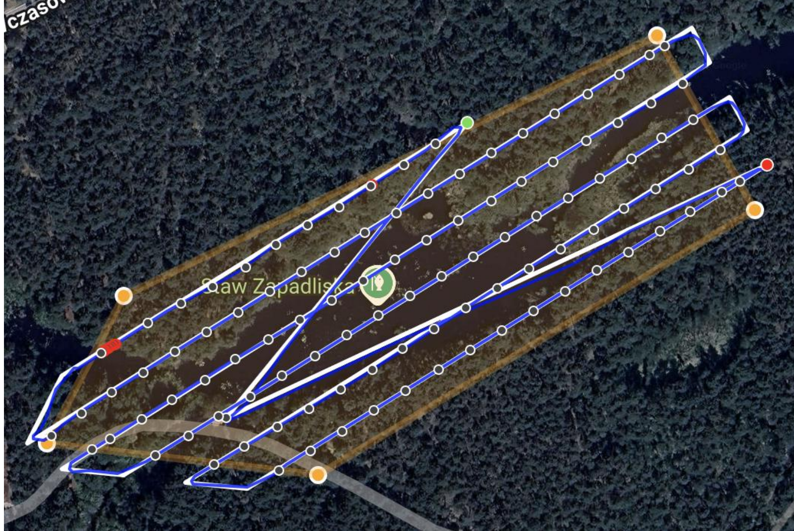
Path of flight lines designed to register orthophoto of Zapadliska Lake
