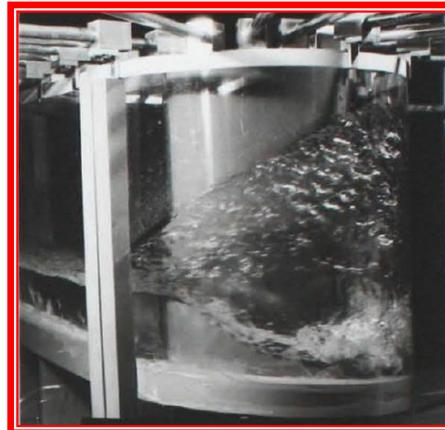
Vortex intake **subcritical** and **supercritical** approach flow
